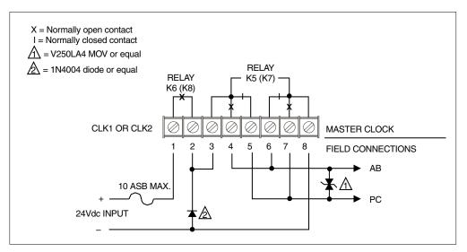
Figure B-19 Two-Wire Minute Impulse (59th Minute) with 12-Hour Correction
